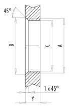
Installation direction: o-ring sits on chamfer.
